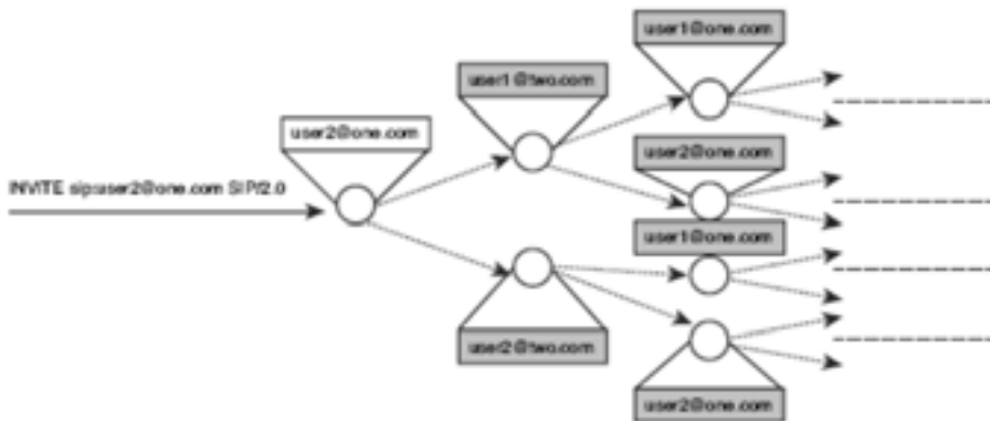
Figura 7 – SIP Signalling Loop
